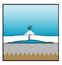
6. If the conditions are right, this insoluble calcium carbonate can build up a "slag pile" around the exit point, thus forming a nodule.
