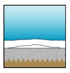
2. Sometimes, an air cavity can be formed between the gunite and the plaster. This is referred to as "delamination" and the cavity is referred to as a "void." As long as the void is not connected to the surface of the plaster, the fact that the void even exists may not be known. Unless the plaster completely breaks free from the surrounding plaster, creating what is referred to as a "pop—off," or unless the delamination is extensive, this is not considered by the plaster industry to be a defect.
