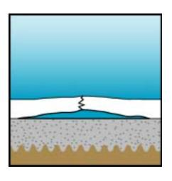
4. Gradually, water from the pool penetrates the void via the hole or crack, and creates a localized chemistry environment completely separate from the water balance in the pool. As calcium hydroxide bleeds into the void water it creates a calcium—rich, high pH solution like a little "calcium/pH factory" beneath the plaster surface. The pinhole or crack is not of sufficient size to create a rinsing effect like that going on at the plaster surface.
