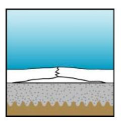
3. In some cases, however, the void is connected to the surface by a small pinhole or hairline crack. Pinholes and cracks are created from structural flexing of the delaminated plaster. The type and size of resulting hole or crack is dependent on numerous factors, including the size and shape of the delamination, the nature of the structural flex, the strength and thickness of the plaster over the delaminated section, etc.
