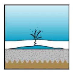
5. Calcium—rich void water and bicarbonate—rich pool water, in contact with each other at the plaster surface, react with each other and seek equilibrium, which results in the production of an insoluble calcium carbonate byproduct.
